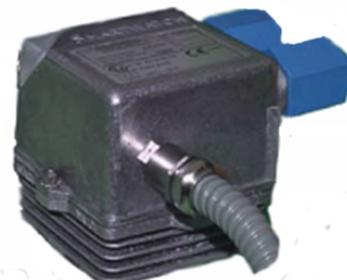
*Valve monitor SWW1X with a pressure sensor connection.*
